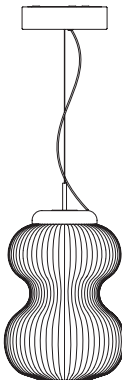
4386.. Ø 31 x 51,3 + 250 cm 13W Led (2700K, CRI>90, 900 Lm) + 4W Led (2700K, CRI>90, 450 Lm)* dimmable
